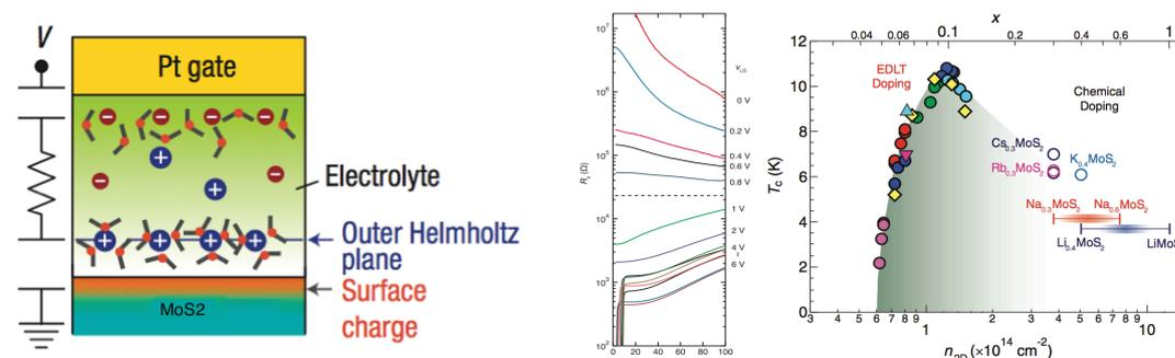
**Fig. 1: Transforming the MoS<sub>2</sub> 2D insulator into a metal.** *Left:* FET device configuration. *Center:* transversal resistivity of the MoS<sub>2</sub> sample changing from insulating to metallic by increasing  $V$ . *Right:* Superconducting phase diagram of MoS<sub>2</sub> by FET doping and intercalation.
