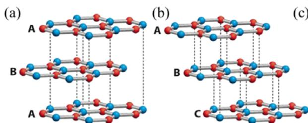
stacking (see stacking ABC in figure (b) below). Two interfacial states form at the top and the bottom surface of the N-multilayer. The ABC coupling make these states have a very low kinetic energy : a flat band with high effective mass. If we populate these states with electrons, we expect the Coulomb
